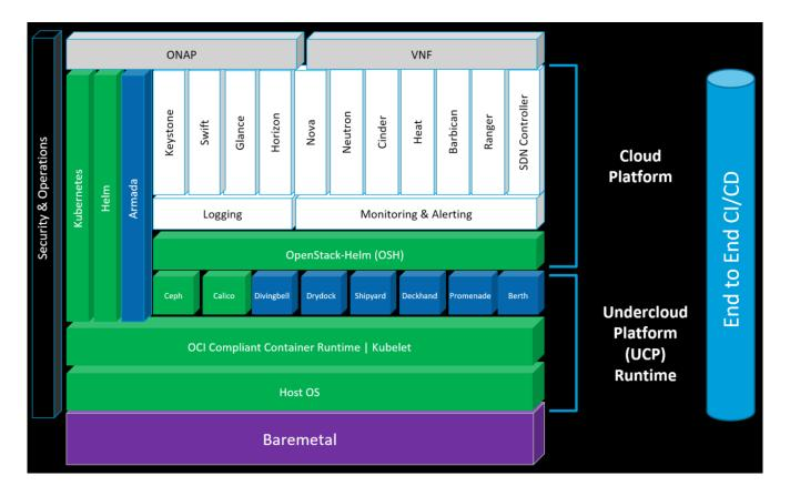
Figure 1 – Software Layers of the AT&T Network Cloud Reference Design
